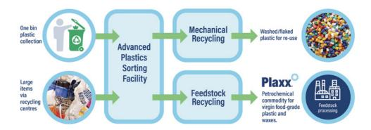
Project Beacon at Binn Ecopark, is a collaboration between the Binn Group, EcoideaM Ltd, Pi Polymer Recycling Ltd and Recycling Technologies Ltd. This group is developing a new concept **Advanced Plastics Recycling Facility** (A-PRF).
